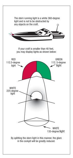
shall display a 225-degree (112.5-degrees on each side of the watercraft) unbroken white light above and forward of the stern light along the center line of the watercraft. The stern light shall display a 135-degree unbroken white light placed as near to the stern as practicable. Separate sidelights showing red 112.5 degrees to port (left) and green 112.5 degrees to starboard (right) shall be used and fitted with screens to prevent them from being seen across the bow.
